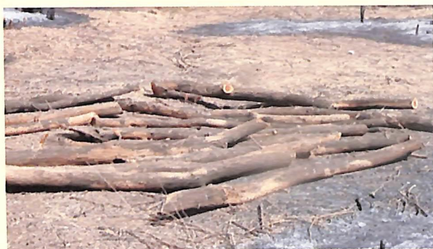
Plate 2. Prosopis poles laid on ground to form kiln base
