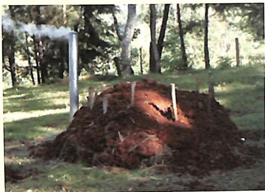
Plate 4. Improved earth kiln emitting smoke through the chimney
